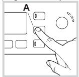
To start the programme press button **A** for 5 seconds (see figure). The programme will start automatically and will run for about 70 minutes. To stop the cycle press the START/ PAUSE button.
